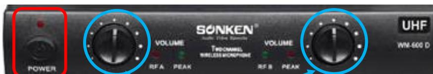
**Step 5** Turn Volume knobs on front panel to half way (no more otherwise you will get feedback/squealing) you will be able to turn the microphone volume up from the device you are plugging it into.
